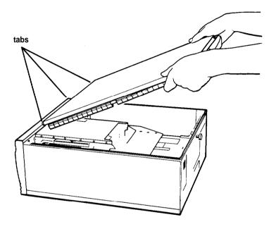
2. Insert the three tabs into the three notches in the back of the front panel of the computer.
